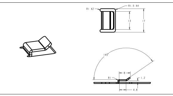
Figure 13. Suggested Mounting Tab (chassis feature)
